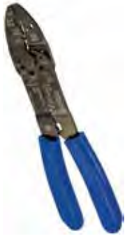
CT-100 (MULTI-TOOL) ECONOMY/STANDARD 22-8 GA INSULATED & NON- INSULATED, SPRING LOADED, ALSO CUTS SMALL SCREWS (LENGTH 8")
